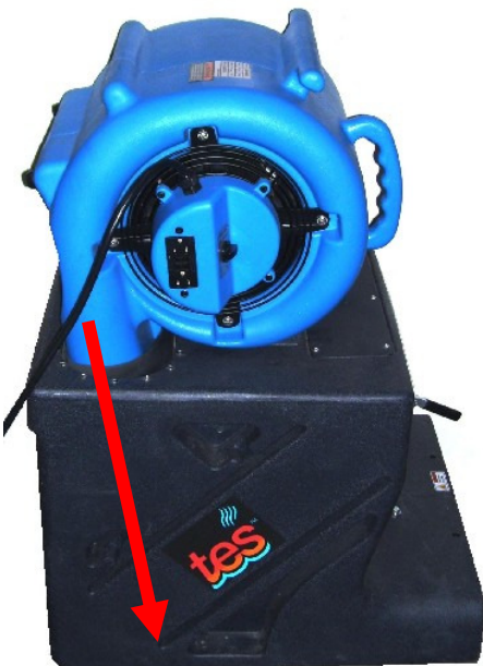
Snout Not Angled Properly
